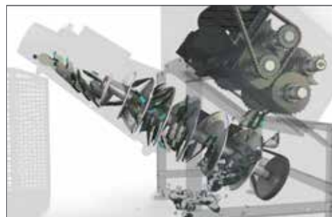
Emptying and compression of the material in one step
